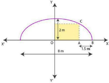
The equation of the semi – ellipse will be of the from  $x^2/16 + y^2/4 = 1$ ,  $y \ge 0$  ... (1 Let A be a point on the major axis such that AB = 1.5m.
