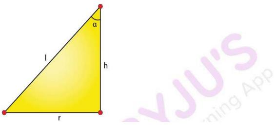
Let r be the radius of the base circle of the cone and I be the slant length and h be the height of the cone
