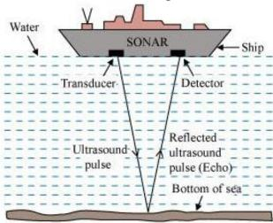
20. A sonar device on a submarine sends out a signal and receives an echo 5 s later. Calculate the speed of sound in water if the distance of the object from the submarine is 3625 m.
