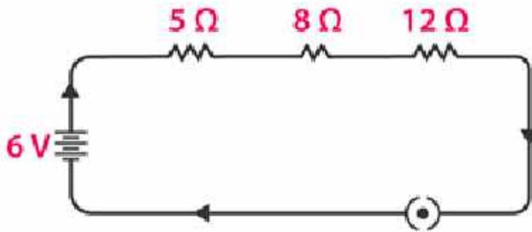
2. Redraw the circuit of Question 1, putting in an ammeter to measure the current through the resistors and a voltmeter to measure the potential difference across the 12 Ω resistor. What would be the readings in the ammeter and the voltmeter?
