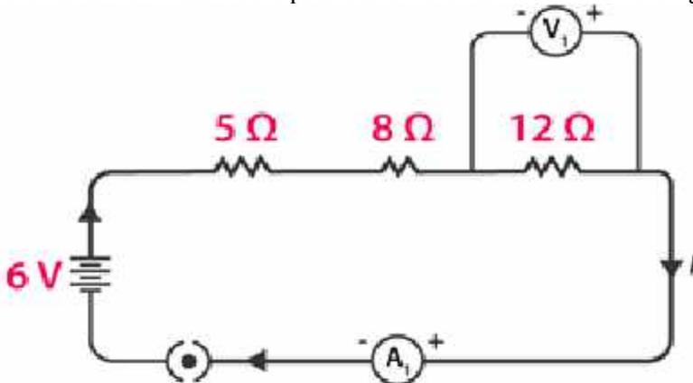
Using Ohm's Law, we can obtain the reading of the ammeter and the voltmeter.
