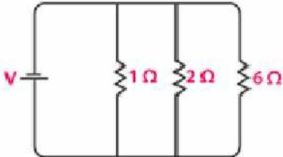
From the circuit, it is understood that all the resistors are connected in parallel. Therefore, their equivalent resistance can be calculated as follows:
