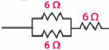
If two resistors are connected in parallel, then their equivalent resistance is
