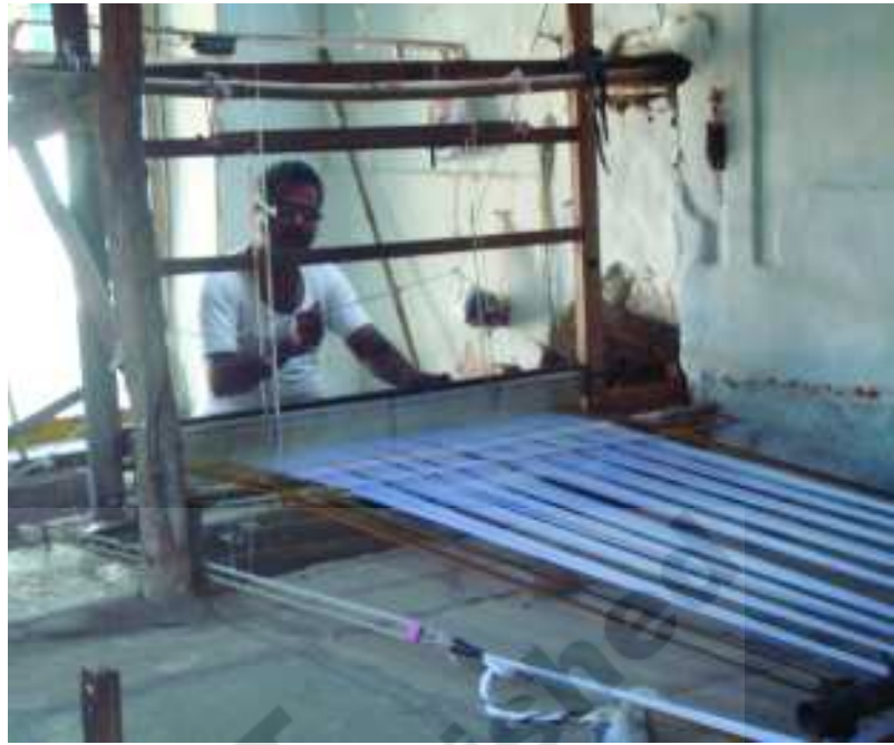
Fig 9.4 At pit loom - weaving a saree
