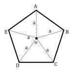
If we assume that q charge is placed at all the 5 corners of the given pentagon then, due to its symmetry, the electric field due to all the charges are cancelled out. As a result of which the electric field at 0 is zero.
