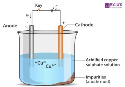
A small electric current is passed through the cell. Atoms from the anode enter the electrolyte. The copper from the anode gets converted into copper sulphide. An equal number of copper atoms from the solution get deposited on the cathode. This is to keep the concentration of the solution constant. Impurities from the anode block either remain in solution or collect below the anode, as they are unable
