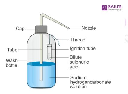
Making a soda-acid fire extinguisher
