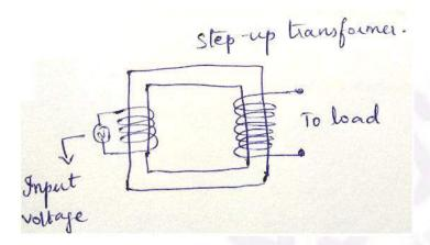
AC voltage  $v_i$  is applied at primary P of transformer (with turns  $N_P$ ).
