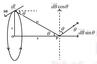
Magnetic field at point P(x, 0, 0) due to  $I \vec{dl}$
