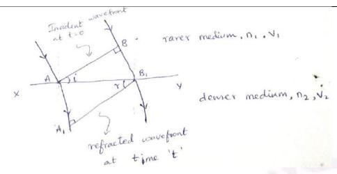
A plane wavefront AB is incident in rarer medium at instant t = 0 on interface XY separating it from a denser medium. When wavelet A is on interface, B is at a distance BB, from it. It takes t time to cover the distance  $BB_1 = v_1t$  to reach on interface XY. Mean while, the wavelet from A reaches to point  $A_1$  covering a distance  $AA_1 = v_2t$  in denser medium.
