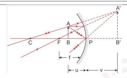
$$\Delta ABC \sim \Delta A_1 B_1 C \Rightarrow \frac{A_1 B_1}{AB} = \frac{A_1 C}{AC} = \frac{(+v) + (-R)}{(-R) - (-u)} \qquad \dots (1)$$
