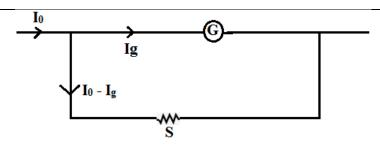
(G) can be converted into an ammeter by connected a small stunt resistance parallel to (G) coil so that
