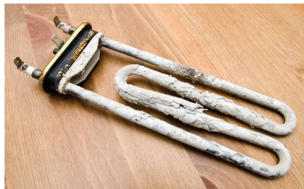
Figure 4.8 Scales on the machine pipes
