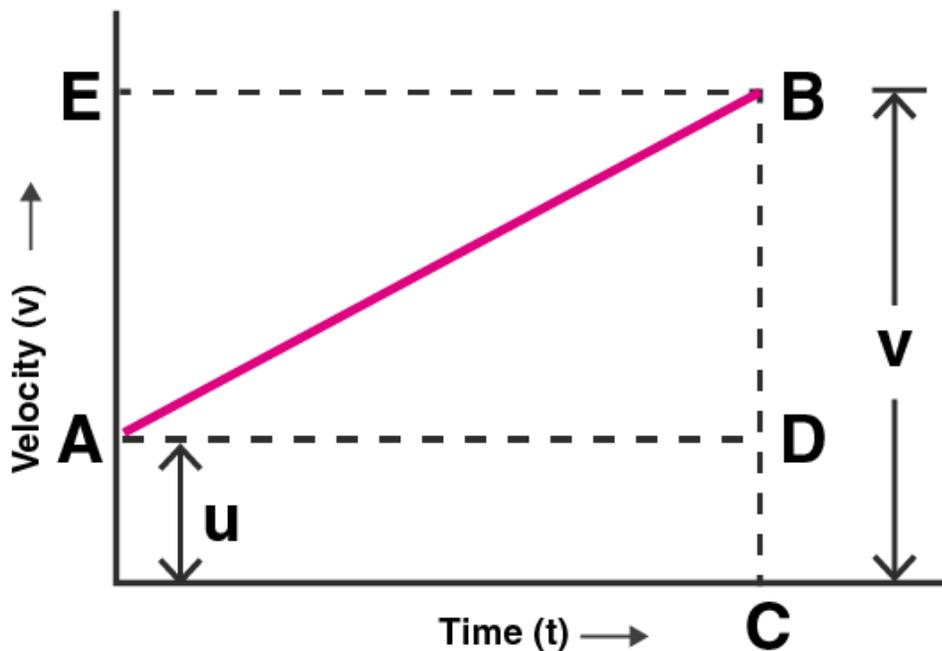
The initial velocity  $u$  at point A changes at a uniform rate from A to B in time  $t$ . BC is the final velocity  $v$  in the graph. The time  $t$  is represented by OC. The distance travelled by the body is the area under the OABC.
