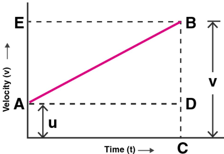
Let  $u$  be the initial velocity at point A such that the velocity changes at a uniform rate from A to B in time  $t$ . Let  $v$  be the final velocity which is BC in the graph. OC in graph represents the time taken  $t$ . CB is the perpendicular that is drawn to complete the figure from point C and AD is drawn parallel to OC. BE is the perpendicular from point B to OE.
