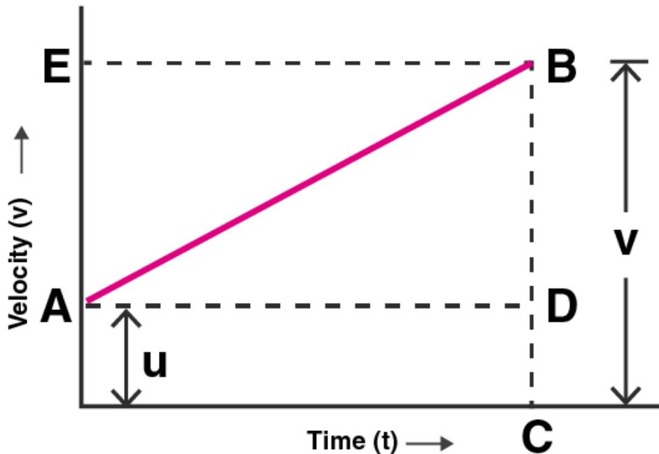
The initial velocity is  $u$  at the point A which changes from A to B at uniform rate in time  $t$ . Let  $v$  be the final velocity which is equal to BC in the graph. OC represents the time  $t$ . A perpendicular is drawn CB from point C and AD is drawn parallel to OC. BE is the perpendicular from point B to OE. The area under OABC is the distance travelled  $s$ .
