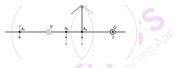
P and Q are the two wires having opposite direction of current.
