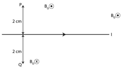
Cross determines the field going into the plane and dot determines the field coming out of the field.
