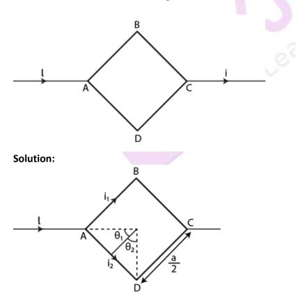
Let  $i_1$  and  $i_2$  currents and r and 2r be the resistances in wires ABC and ADC,  $i_1/i_2 = 2/1$
