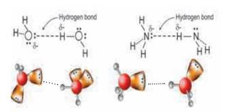
Fig. 10.4 : H-bonding in  $H_2O$  (above) and  $NH_3$  (below) (solid line denotes covalent bond, dotted line denotes hydrogen bond)
