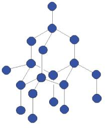
Fig 9.1 Structure of diamond
