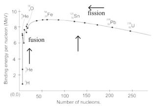
Fig. 13.2 : Binding energy per nucleon
