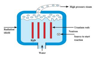
Fig. 13.4 (a) : simplified nuclear reactor
