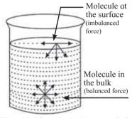
Fig. 10.18 : Imbalance of forces at the surface of a liquid
