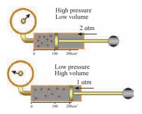
Fig. 10.7 : Schematic of the experiment Boyle's law
