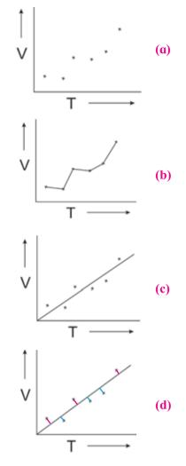
Fig. 2.2 : Drawing an average curve through the points on graph
