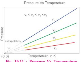
Fig. 10.11 : Pressure Vs Temperature graph of a gas
