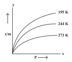
Fig 11.2 Variation of adsorption with temperature and pressure
