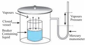
Fig. 10.17 : Vapour pressure of a liquid
