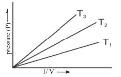
c. Graph of pressure, P, of a gas vs 1/V at different temperatures  $T_1, T_2, T_3$ .
