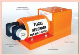
string to encode the data; these days they use solid-state memory boards. Solid-state recorders in large aircraft can track more than 700 parameters.
