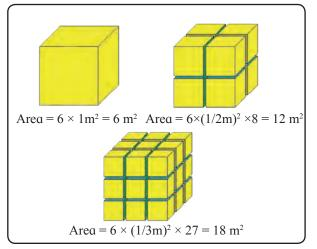
Fig. 16.5 : Surface area of nanoparticles
