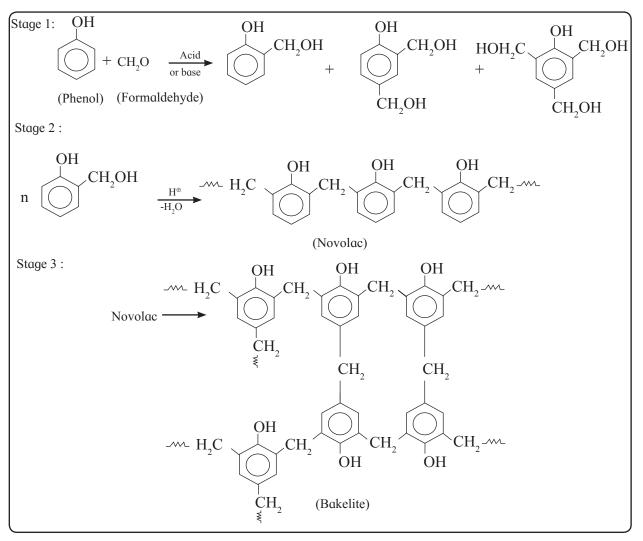
Fig. 15.3 Preparation of Bakelite
