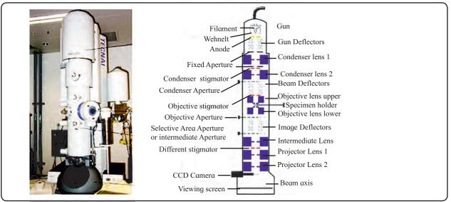
Fig. 16.11Transmission electron microscope (TEM)
