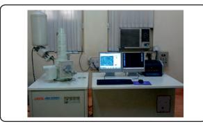
Fig. 16.10 Scanning electron microscope
