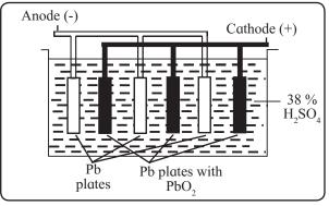
Fig. 5.9 : Lead storage cell
