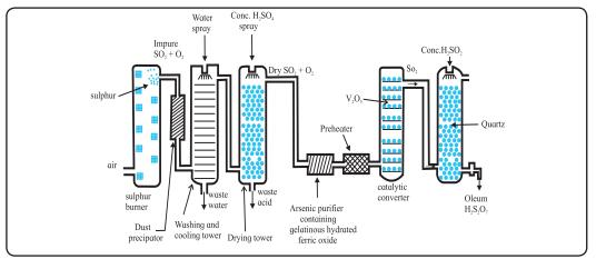
Fig. 7.1 : Flow diagram for manufacture of Sulfuric acid
