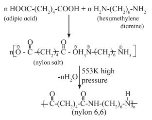
The numerals 6,6 in the name of this polymer stand for the number of carbon atoms in the two bifunctional monomers, namely, adipic acid and hexamethylenediamine.
