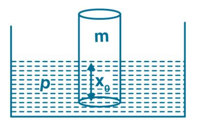
The SHM executed by the cylindrical wood log is given as  $T = 2\pi \sqrt{m/A\rho g}$
