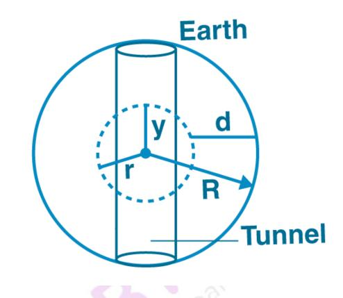
Acceleration due to gravity of the earth inside the earth is g' g' = g(1-d/R) R-d = y g' = g y/R F = -mg y/R F is proportional to (-y) When the body is in a tunnel the motion is SHM. ma = -mg'  $T = 2\pi \sqrt{R/g}$
