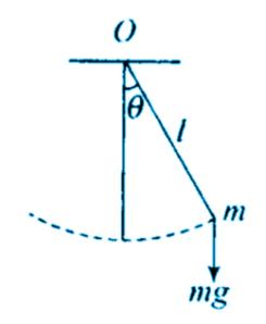
Consider a simple pendulum with O as the fixed point that has a restoring torque. The restoring force is given as  $F = -mg \sin \theta$  $\theta$  is so small that  $\theta = arc/radius = x/l$ Therefore, F = -mg x/lTherefore, it can be said that the motion of the simple pendulum will be simple harmonic when  $\theta$  is small.
