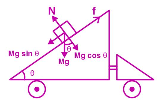
From the above figure it is clear that the block is inclined on the plane. There is no work done, as there is no displacement happening and no dissipation energy takes place.
