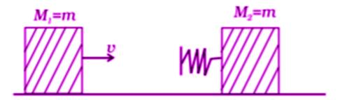
a) while spring is fully compressed all the KE of M1 is stored as PE of spring
