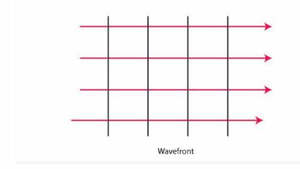
(iii) When the light is coming from a distant star that is intercepted by the earth, the shape of the wavefront is plane.
