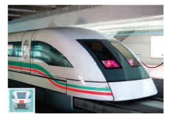
Magnetic levitation (Maglev) is a method by which an object is suspended with no support other than magnetic fields. In maglev trains two sets of magnets are used, one set to repel and push the train up off the track, then another set to move the floating train ahead at great speed without friction. In this technology, there is no moving part. The train travels along a guideway of magnets which controls the train's stability and speed using the basic principles of magnets.
