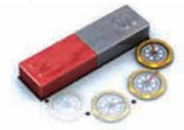
Figure 3.3 Compass showing direction of magnetic field
