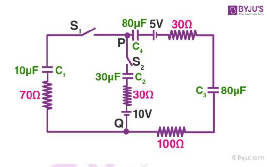
(a) At time t = 0, the S<sub>1</sub> is closed instantaneous current in the closed circuit will be 25 mA
