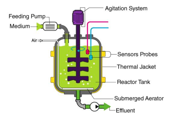
Flask is used to small laboratory scale testing of culture and bioreactor is used for commercial-scale production.
