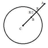
$$V_{A} = \frac{KQ}{(2R)^{2}} - \frac{K\alpha Q}{R^{2}} = \frac{KQ}{4R^{2}} - \frac{\alpha V_{0}}{R}$$
