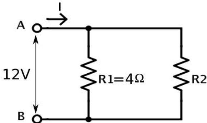
A student has two resistors-  $2\ \Omega$  and  $3\ \Omega$ . She has to put one of them in place of  $R_2$  as shown in the circuit. The current that she needs in the entire circuit is exactly  $9\text{A}$ . Show by calculation which of the two resistors she should choose.
