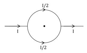
Net magnetic field at the centre will be zero, as the magnitude of the magnetic field due to each half circle will be same but opposite in direction.
