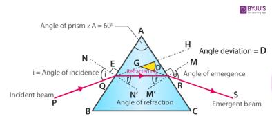
Tracing the path of light ray through prism
