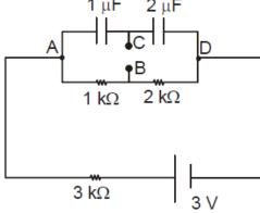
Consider the circuit given here. The potential difference  $V_{BC}$  between the points B and C is
