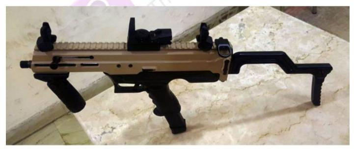
• The Asmi machine pistol fires the in-service 9 mm ammunition and has an upper receiver made from aircraft-grade aluminium and lower receiver from carbon fibre.
