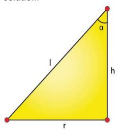
Let r be the radius of the base circle of the cone and l be the slant length and h be the height of the cone
