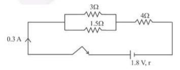
The diagram above shows three resistors connected across a cell of e.m.f. 1.8 V and internal resistance r. Calculate:
