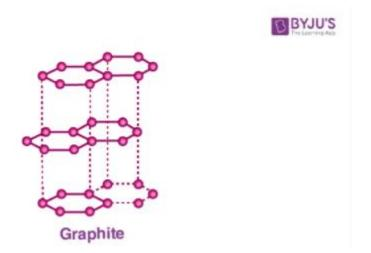
It has hybridized carbon sp<sup>2</sup>, structured in layer form. These layers are held together by the forces of weak van der Walls. These layers may slide over each other, making graphite slippery and soft. Consequently, it is used as a lubricant.
