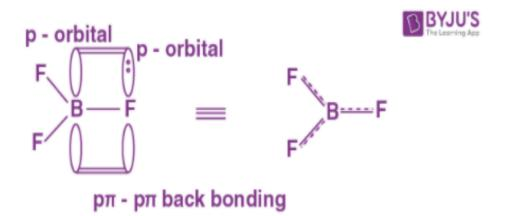
This double-bond character causes a shortening of the bond length by  $BF_3$  (130 pm). However, a change in hybridization from sp.<sup>2</sup> (in  $BF_3$ ) to sp<sup>3</sup> (in  $BF_4^-$ ) occurs when  $BF_3$  coordinates with the fluoride ion. Boron now forms 4 bonds and the character of the double-bond is lost. This represents the length of a 143 pm B-F bond in  $BF_4^-$  ion.
