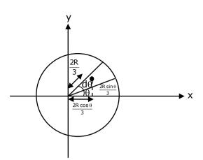
Each segment of disc subtending angle  $d\theta$  can be considered as a triangle of height R and base Rd $\theta$
