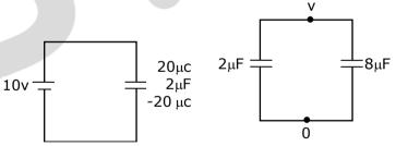
When battery is removed & the capacitor is connected
