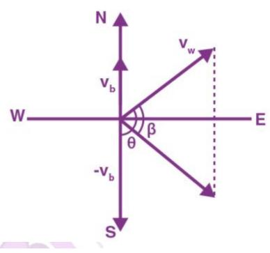
The angle between  $v_w$  and  $(-v_b)$  =  $90^\circ+~45^\circ$   $aneta=~rac{51\sin(90+45)}{72+51\cos(90+45)}$
