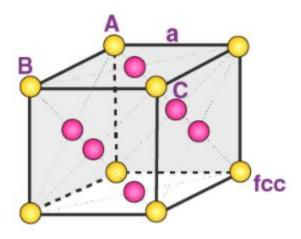
Let the edge length of the unit cell = a let the radius of each sphere = r Thus, AC = 4r From the right angled triangle ABC, we have:  $AC = (a^2 + a^2)^{1/2} = a(2)^{1/2}$
