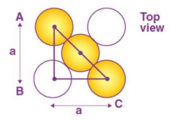
Therefore,  $4r = a(2)^{1/2}$ =>  $a = 4r/(2)^{1/2}$ Thus, Volume of unit cell = $a^3 = \{4r/(2)^{1/2}\}^3$  $a^3 = 64r^3/2(2)^{1/2} = 32r^3/(2)^{1/2}$ No. of unit cell in FCC = 4 Volume of four spheres =  $4 \times \pi r^3(4/3)$
