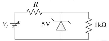
The value of R and the minimum required power dissipation rating of the diode, respectively, are
