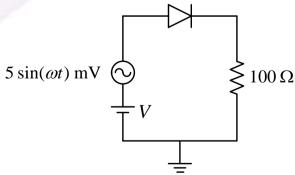
For  $\omega = 2 \times 10^6$  rad/s, the amplitude of the small-signal component of diode current (in  $\mu A$ , correct to one decimal place) is \_\_\_\_\_.
