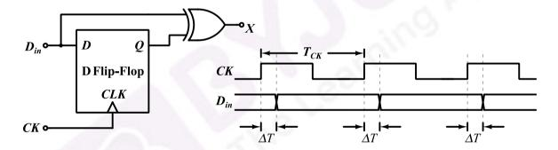
If the probability of input data bit  $(D_{in})$  transition in each clock period is 0.3, the average value (in volts, accurate to two decimal places) of the voltage at node X, is \_\_\_\_\_\_.
