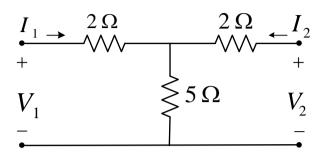
The parameter B for the given two-port network (in ohms, correct to two decimal places) is
