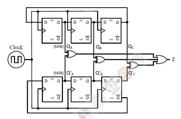
The minimum number of clock cycles after which the output Z would again become zero is
