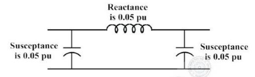
If this transmission line is removed from service, what is the modified bus admittance matrix?
