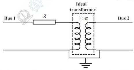
For the given circuit,  $Y_{bus}$  and  $Z_{bus}$  are bus admittance matrix and bus impedance matrix, respectively, each of size  $2 \times 2$ . Which one of the following statements is true?
