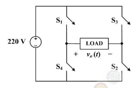
The RMS value of the fundamental component of  $v_o(t)$  in volts is \_\_\_\_\_.
