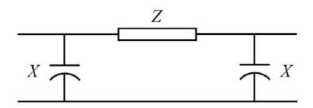
Impedance  $Z = 100 \angle 80^{\circ} \Omega$  and reactance  $X = 3300 \Omega$ . The magnitude of the characteristic impedance of the transmission line, in  $\Omega$ , is \_\_\_\_\_\_. (Give the answer up to one decimal place.)
