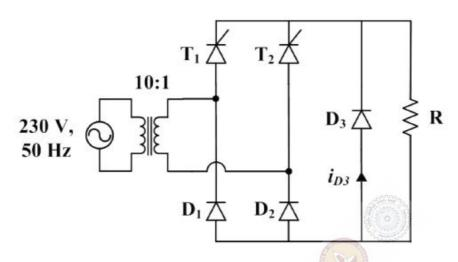
The RMS value of the current through diode D<sub>3</sub> in amperes is
