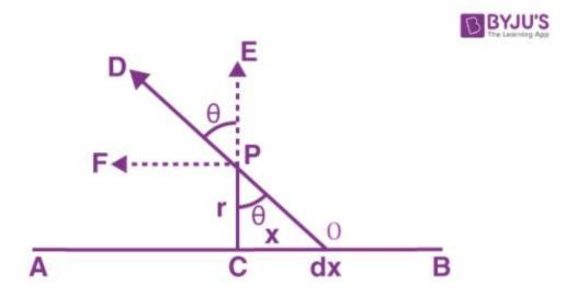
Consider a long thin wire of uniform linear charge density  $\lambda$ . A point P is taken at a distance r from the midpoint C of the wire. The electric field at a point P due to the wire is E.
