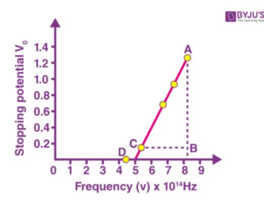
The graph is a straight line. It intersects the y-axis at 5 x  $10^{14}$  Hz. This is the threshold frequency. The point D is the frequency less than the threshold frequency.
