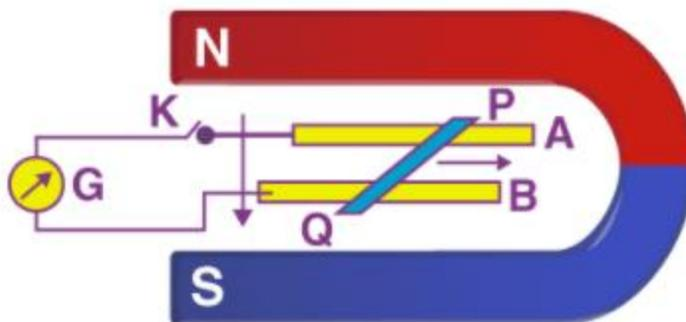
(i) Determine the polarity and the magnitude of the induced emf if we will keep the K open and the rod will be moved with the speed of 12 cm/s in the direction shown in the figure.
