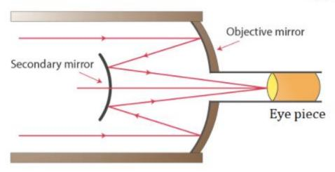
Distance between the objective mirror and the secondary mirror, d = 20 mm
