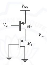
Ignoring the body effect, the ac small signal voltage gain  $(\partial V_{out}/\partial V_{in})$  of the circuit is
