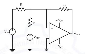
Assuming  $|V_{IN}| \ll |V_{CC}|$  and  $|V_{REF}| \ll |V_{CC}|,$  the condition at which  $V_{OUT}$  equals to zero is
