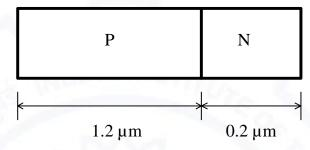
The magnitude of reverse bias voltage that would completely deplete one of the two regions (P or N) prior to the other (rounded off to one decimal place) is \_\_\_\_\_\_ V.
