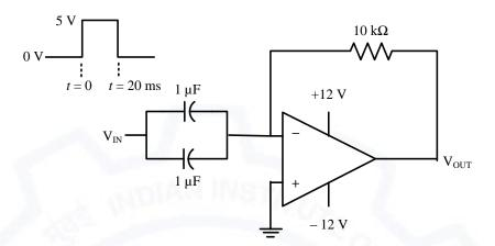
The output voltage  $V_{OUT}$  of this circuit at  $t = 0^+$  (in integer) is \_\_\_\_\_\_V.
