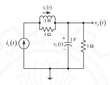
Current  $i_L(t)$  in the inductor and voltage  $v_C(t)$  across the capacitor are taken as the state variables, both assumed to be initially equal to zero, i.e.,  $i_L(0)=0$  and  $v_C(0)=0$ . The system is
