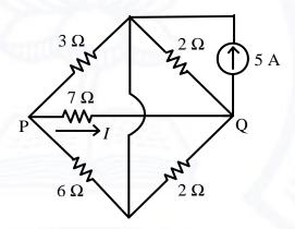
The current I flowing through the 7  $\Omega$  resistor between P and Q (rounded off to one decimal place) is \_\_\_\_\_ A.
