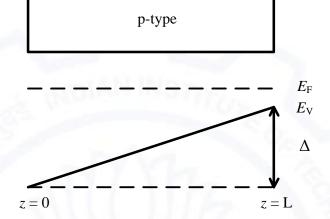
If the charge of an electron is q, then the magnitude of the electric field developed inside this semiconductor bar is
