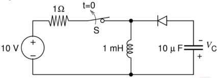
The steady state magnitude of the capacitor voltage  $V_{\rm C}$  (in volts) is
