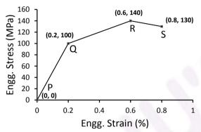
The toughness of the material (in MJ/m<sup>3</sup>) is \_\_\_\_\_
