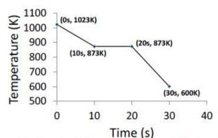
Assuming uniform temperature throughout the volume of the metal during solidification, the latent heat of fusion of the metal (in kJ/kg) is \_\_\_\_\_
