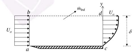
The ratio of the mass flow rate,  $\dot{m}_{bd}$ , leaving through the horizontal section b-d to that entering through the vertical section a-b is \_\_\_\_\_
