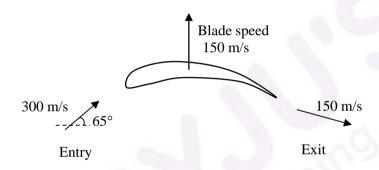
The magnitude of absolute velocity at entry is 300 m/s at an angle of 65° to the axial direction, while the magnitude of the absolute velocity at exit is 150 m/s. The exit velocity vector has a component in the downward direction. Given that the axial (horizontal) velocity is the same at entry and exit, the specific work (in kJ/kg) is\_\_\_\_\_\_
