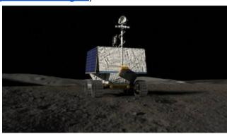
• The size of the lunar rover is approximately the same as a golf cart, with dimensions 5 feet by 5 feet by 8 feet and a weight of 430 kilograms
