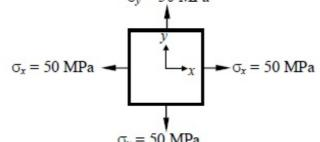
(A) -50 MPa, on a plane 45<sup>0</sup> clockwise w.r.t. x-axis
