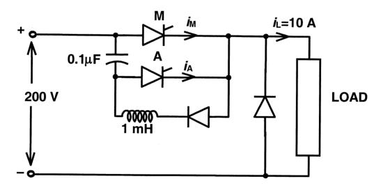
If the maximum value of load current is 10 A, then the maximum current through the main (M) and auxiliary (A) thyristors will be
