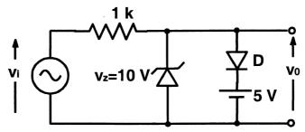
Assuming forward voltage drops of the diodes to be 0.7 V, the input-output transfer characteristics of the circuit is
