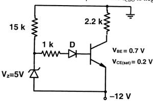
If the forward voltage drop of diode is 0.7 V, then the current through collector will be
