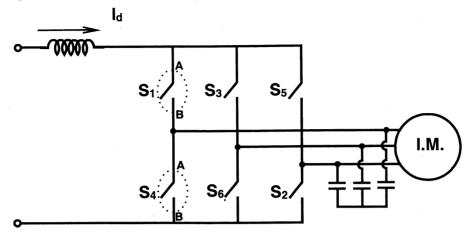
The proper configuration for realizing switches  $S_1$  to  $S_6$  is
