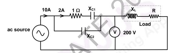
The voltmeter, across the load, reads 200 V. The value of  $X_L$  is \_\_
