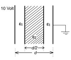
If the potential difference between one of the plates and the nearest surface of dielectric interface is 2 Volts, then the ratio  $\varepsilon_1$ :  $\varepsilon_2$  is
