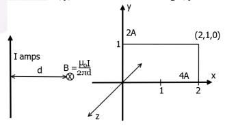
Assuming right handed coordinate system, magnetic field intensity,  $\vec{H}$  at coordinate (2,1,0) will be
