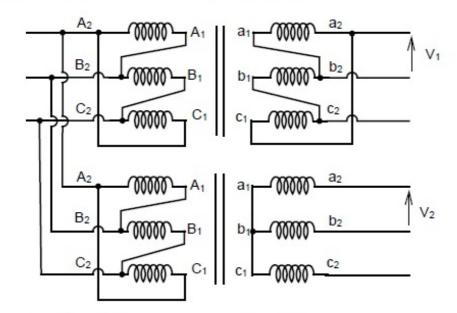
The phase difference (in degree) between voltages V<sub>1</sub> and V<sub>2</sub> is \_\_\_\_\_\_.
