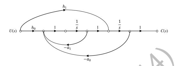
Assuming,  $h_1 = b_1$  and  $h_0 = b_0 - b_1 a_1$ , the input-output transfer function, G(s) =of the system is given by
