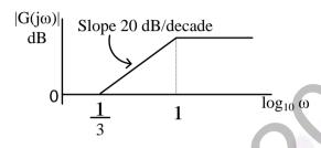
The maximum phase angle  $\phi_m$  and the corresponding gain  $G_m$  respectively, are
